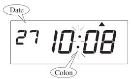
Push the <u>SETTING END</u> button to get out of the setting mode.
