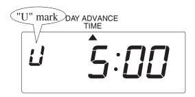
"U" mark is indicated on the left-side of display, and you can not change setting with control buttons on the unit.
