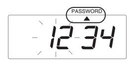
Position the "\[ \Lambda " under the "PASSWORD" mark. At that moment, the first two digits "12" flash.
